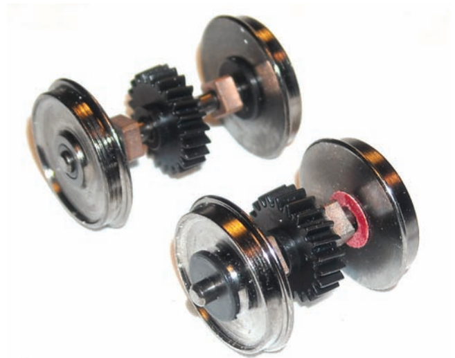
Top is the original wheelset and below is a reassembled and regauged wheelset for On30. Please note that the plastic axle hub must be installed reversed from its original configuration. This is to provide enough clearance with the truck frame.
