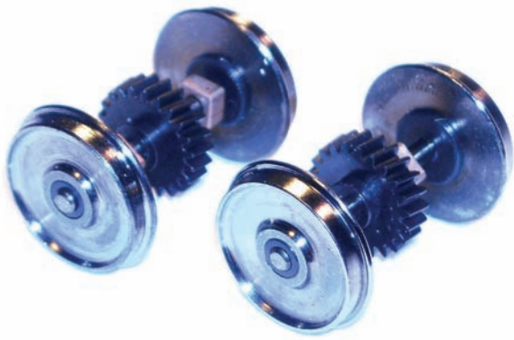
Here is the scale wheelsets provided with the S scale SW-1
