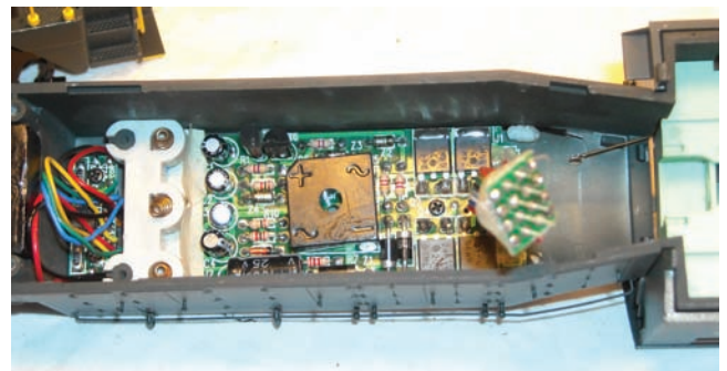
AC electronics which are not needed and can be removed. Some are glued in some are held by screws.
